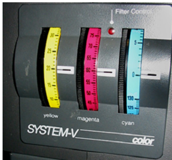
Filter dials on a colour enlarger yellow magenta cyan. Traditional photography might use increments to 25 cc - for the photograms increments up to 130
